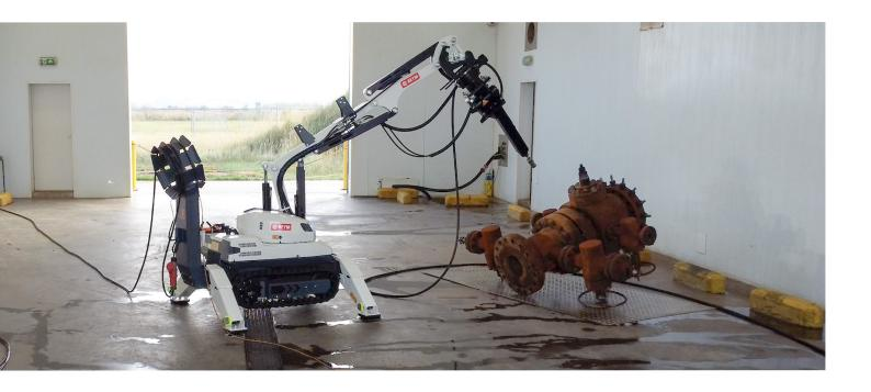
The Multibot is an advanced robotic system designed to perform extended, demanding tasks, particularly on cleaning yards during large-scale shutdowns. By utilizing the Multibot, our employees can operate outside the "line of fire," significantly enhancing safety and reducing exposure to risks. This state-of-the-art robot is capable of both high-pressure and vacuum operations.
